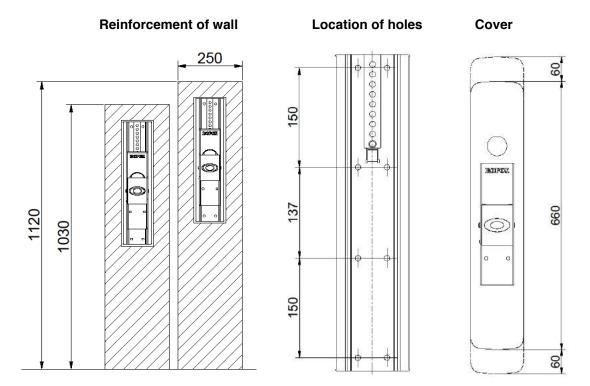
The hatched area is the minimum area for reinforcement of the wall. Reinforcement from floor to ceiling is advisable. The holes are measured on the basis of the upper holes of the wall bracket and the location depends of the type of toilet support arm to be used. It must be ensured that the cover can move 60mm upward and downward.
