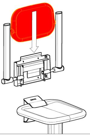
Please note: Mount only the PUR backrest under tempered conditions. At 10  $\,\mathrm{C}^{\circ}$  or lower the backrest surface could crack during mounting.
