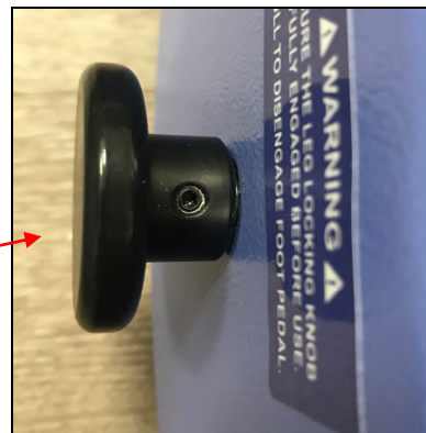
Fig. 2 Close up of leg locking knob and accompanying warning decal.
