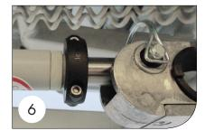
**4.** The clamping device is now loosely mounted. **5.** Lower the bed to its lowest position. Raise the bed again to make space for working. Bring the clamping device 4 mm closer to the actuator housing. Tighten the clamping device well. **6.** Test the installation while making sure functions work. Run 5 times with the bed against the stop for further testing.
