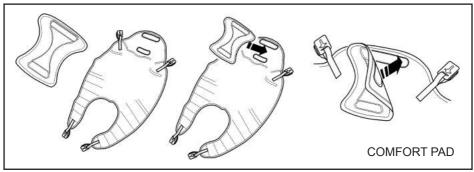
The Comfort Pad must be applied as it provides additional comfort and support to the client. **Do not** lift without the Comfort Pad correctly in position. The Comfort Pad is available in different thicknesses providing increased levels of support/comfort.
