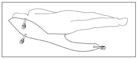
Draw sheet roll the client onto the sling, ensuring that the top of the commode aperture is at the base of the spine. Position the spreader bar as shown opposite and the client is ready for lifting.
