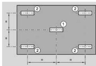
The mounting plate must be at least 10 mm thick.
