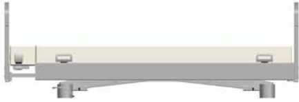
Without a safety side, no additional parts are required, a panel piece is available as an option to fill the gap.
