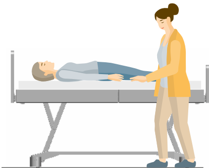
▲ Depending on the model variant, the highest position is between 80 and 85 cm, – i.e. at hip height and therefore ideal for back-friendly work.
