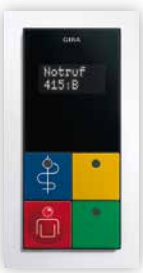
A visual and acoustic signal is activated in the care room.
