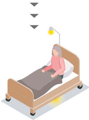
The automatic light system is activated automatically as soon as the resident sits up in bed.
