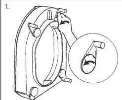
Undo the four fixing screws by turning them anticlockwise. The screws should be loosened only.
