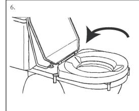
Attach the Hi-Loo to the bowl, front brackets first. Then use downward pressure to secure the rest of the Hi-Loo to the bowl. Check it is securely attached.
