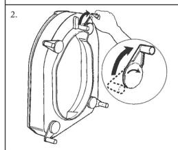
Then move the four brackets towards the outside of the seat. The screws will tighten until they click into place.
