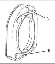
A) Fixing screw (covered in friction rubber)
