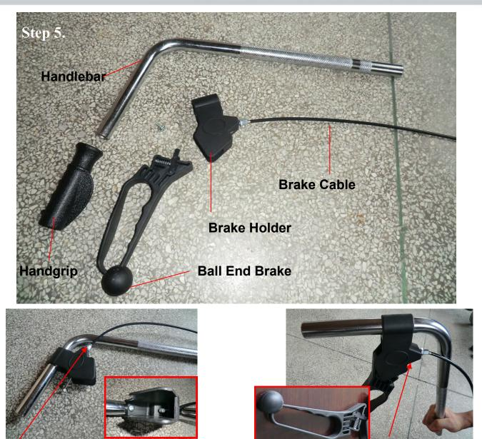
1. Place brake holder into handlebar and tighten the screw
