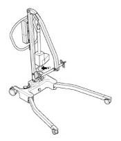
2. Release leg-locking device (pulling it away from the cast base), close legs tightly together.
