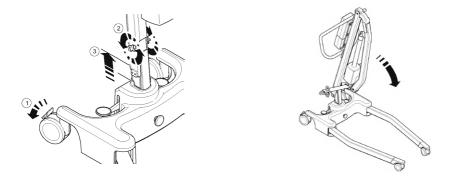
**4.** Lift the folded Advance upright (using the legs and push handle as a guide) being careful that the mast and boom stay together as you tilt upright.
