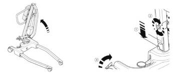
**5.** Open legs fully. ENSURE leg-locking knob engages flush against the base casting and the legs will no longer move freely. The legs will then only operate by the use of the foot pedal mechanism located at the rear of the base.
