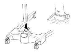
Tighten the mast assembly with the mast-locking device, which is located at the front of the chassis.
