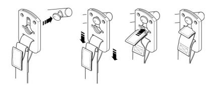
Securi3 sling attachment system. Example of installation.
