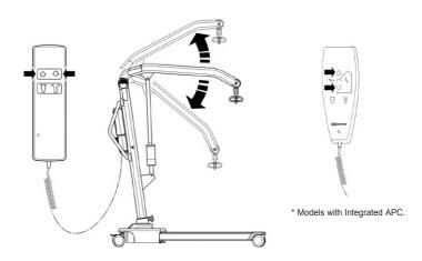
• On models with Integrated APC, push the seated person buttons on the hand control and confirm the cradle re-positions accordingly.
