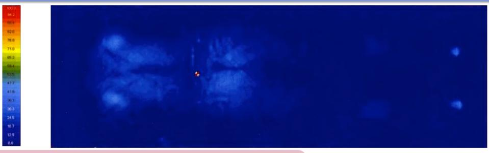
The pressure map is for a **100kg male subject** lying on their back on the Pressure Relieving Mattress designed for Frail users (for users up to 100kg). The map shows the % peak pressure under 50mmHg was 100% and when lying on their side was 99%.
