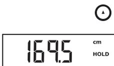
1. Briefly press the arrow key (**hold/zero**), after you have positioned the head slide.
