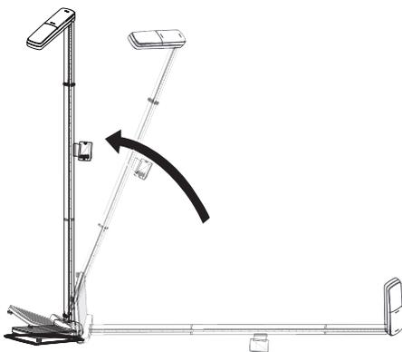
1. Carefully return the device to an upright position.
