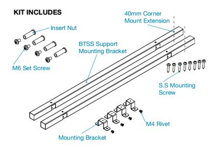
The Mounting Kit for Shower Seats is to assist in the installation of Bendtech<sup>™</sup> Shower Seats where stud spacing may cause mounting issues.
