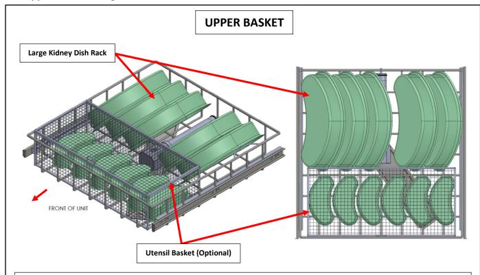
The upper basket is split into two sections, a rack in the rear half for kidney dishes from 160-300mm. And a front section which can accommodate smaller bowls, gallipots and receivers. An optional utensil basket can also be used for smaller items.
