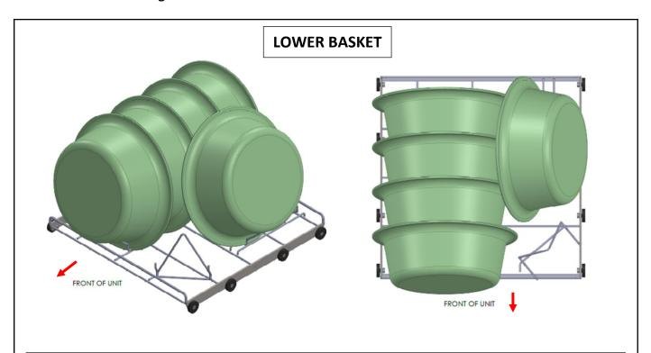
Bowls, dishes, or receivers of 185mm - 345mm in diameter with a depth not greater than 120mm can be loaded in the lower basket as per the above configuration
