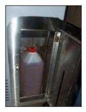
2. Remove empty detergent bottle, unscrew the lid and remove the tube.
