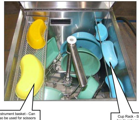
Instrument basket - Can also be used for scissors and knives, must be face down,
