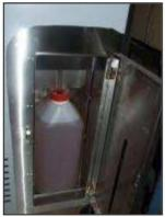
4. Fit bottle cap with tube attached to the full detergent bottle
